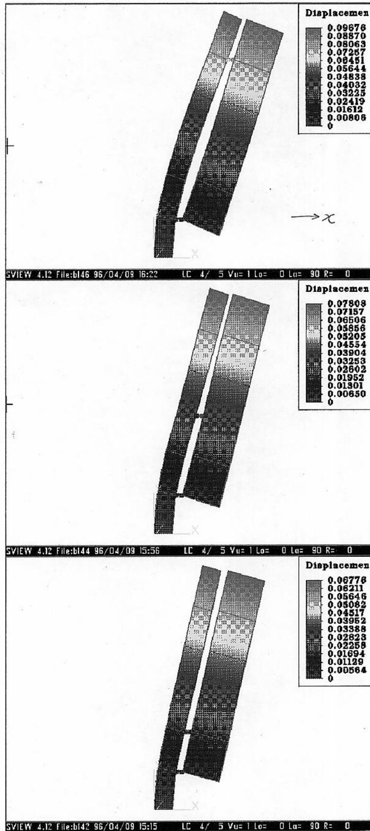
Figure 1: Finite-element analysis of a joint between an aluminum plate tilted by 26 mrad and a 2.5-mm-thick aluminum plate.
