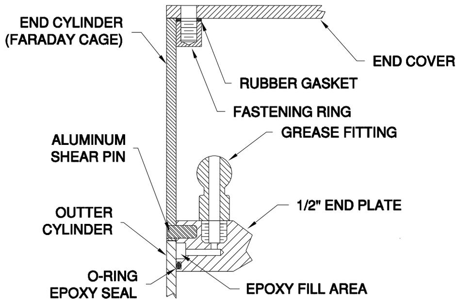
Figure 2: Sketch of the joint between the front endplate and 2.5-mm-thick outer support tube. A 2.5-mm-thick aluminum end cylinder is pinned to the endplate by at least 16 aluminum dowels to support the wire load during gluing. The glue is introduced into a slot in the outer edge of the endplate via several channels that can temporarily be connected to grease fitting. An O-ring in the endplate between the glue channel and the inside of the chamber prevents glue from seeping into the chamber.
