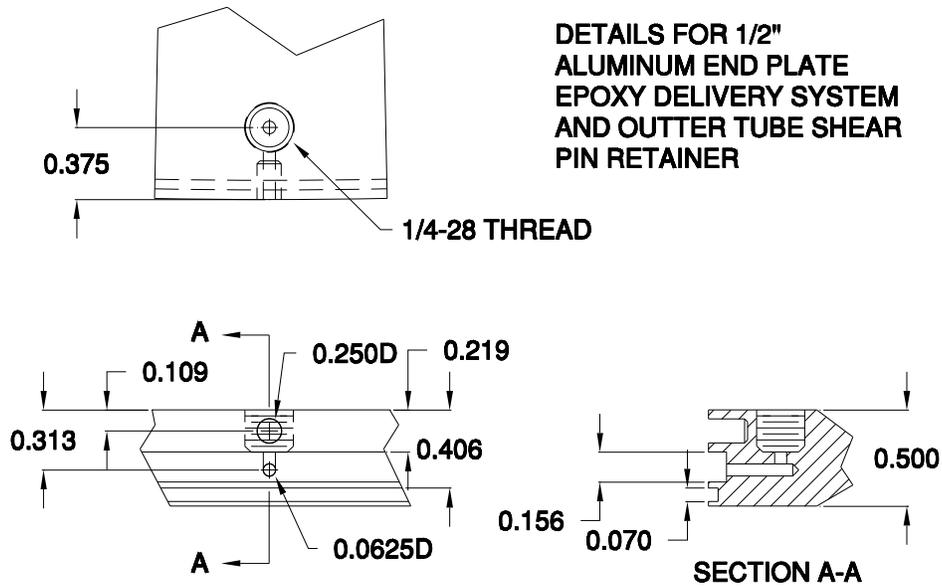
Figure 3: Some details to the proposed glue channels in the endplates.
