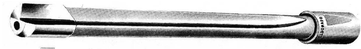
Figure 1: A gun-drill bit showing the hole in the tip for the coolant oil and the V-groove for chip removal.
