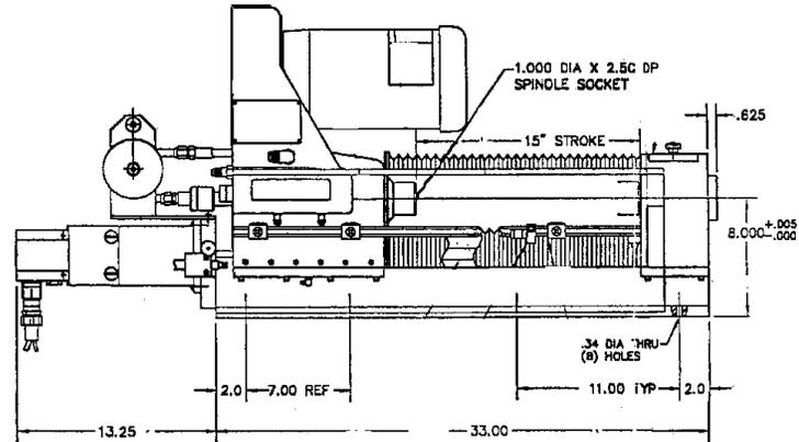
Figure 7: Sketch of the gun-drill machining head sold by Eldorado.
