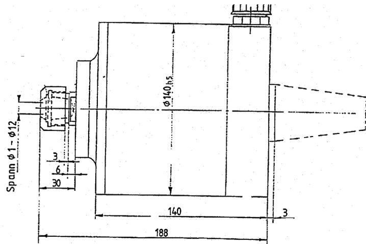
Figure 8: Sketch of a compact 30,000-rpm, 2.5-kW spindle manufactured by Setco/Whitnon.
