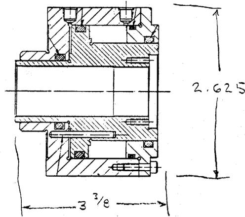
Figure 5: Sketch of an air cylinder to position the bushing against the work-piece.
