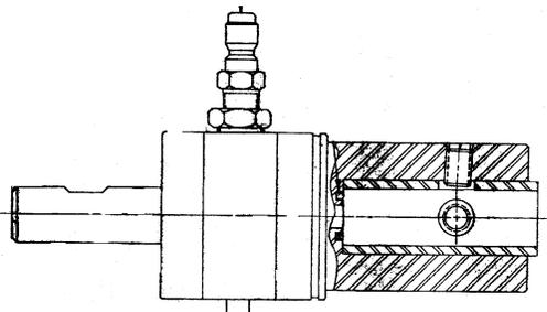
Figure 6: Sketch of a rotary gland that induces 1500 psi cooling into the shaft of a spindle rotating at 10,000 rpm. The shaft at the left is mounted in the spindle, and the gun-drill-bit driver mounts in the shaft to the right.
