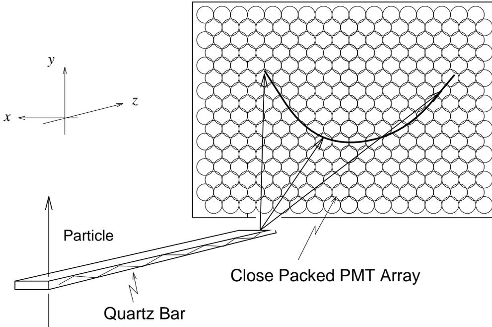
Figure 1: The principle of the DIRC.
