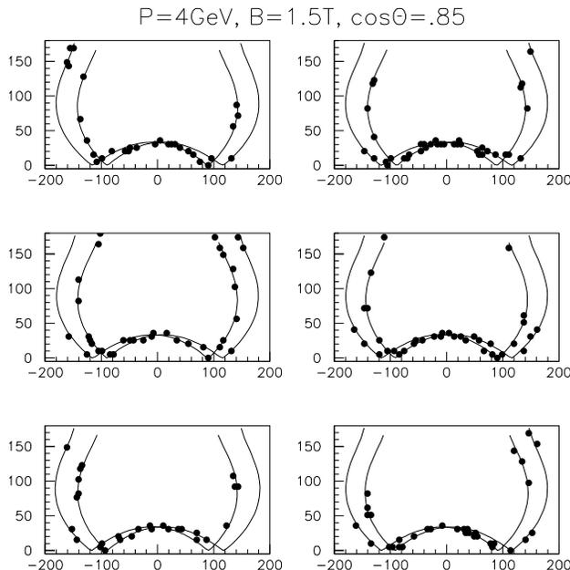
Figure 2: Simulated phototube hit patterns in the BABAR DIRC, along with best-fit ‘hyperboloids’. The ‘hyperboloids’ are folded by reflections at the four walls of the DIRC bar and by the mirror in the water standoff box. They are also distorted by the curved surface of the PMT array.
