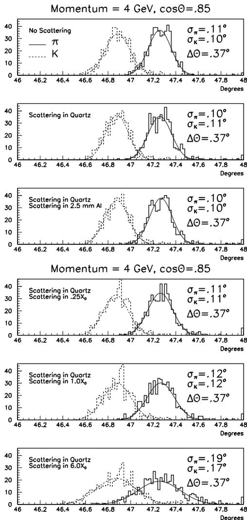
Figure 3: Simulated resolutions in the reconstructed Čerenkov angle for 4-GeV  $\pi$ 's and  $K$ 's entering the DIRC at polar angle  $\cos\theta = 0.85$  for various amounts of multiple scattering in material just in front of the DIRC.
