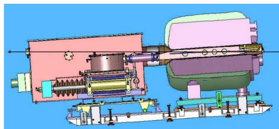
Figure 4: Cutaway view of the high-power-target experiment.
