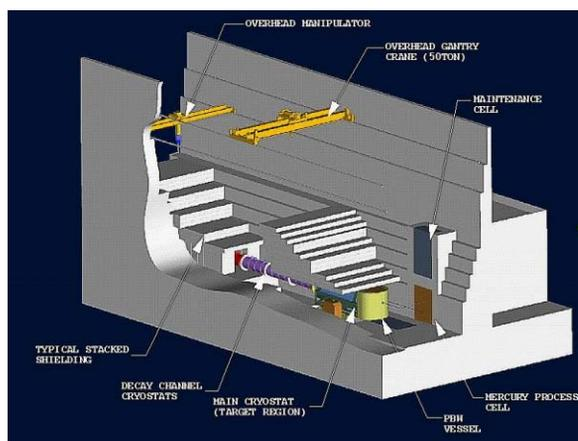
Figure 2: Concept of the target vault for a 4-MW mercury jet target [3].
