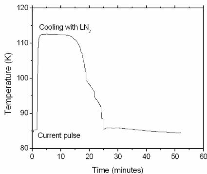
**FIGURE 7.** Magnet cryostat average temperature evolution for a cooling cycle after a 15 T pulse.
