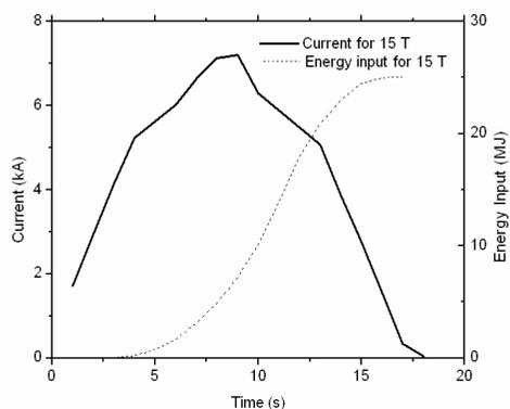
**FIGURE 2.** A magnet pulse of 15 T by ramping the current up and down. During the current plateau the beam intercepted the Hg jet. Energy deposition reached a maximum of 25 MJ.
