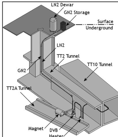
**FIGURE 3.** Layout of the cryogenic system.
