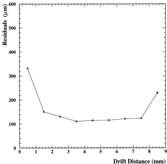
Fig. 3. Prototype II space resolution as a function of the track drift distance from the wire.
