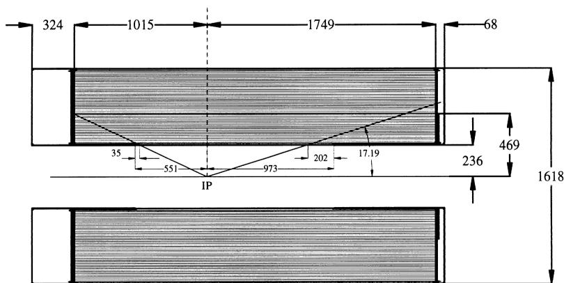
Fig. 1. Layout of the BaBar drift chamber.
