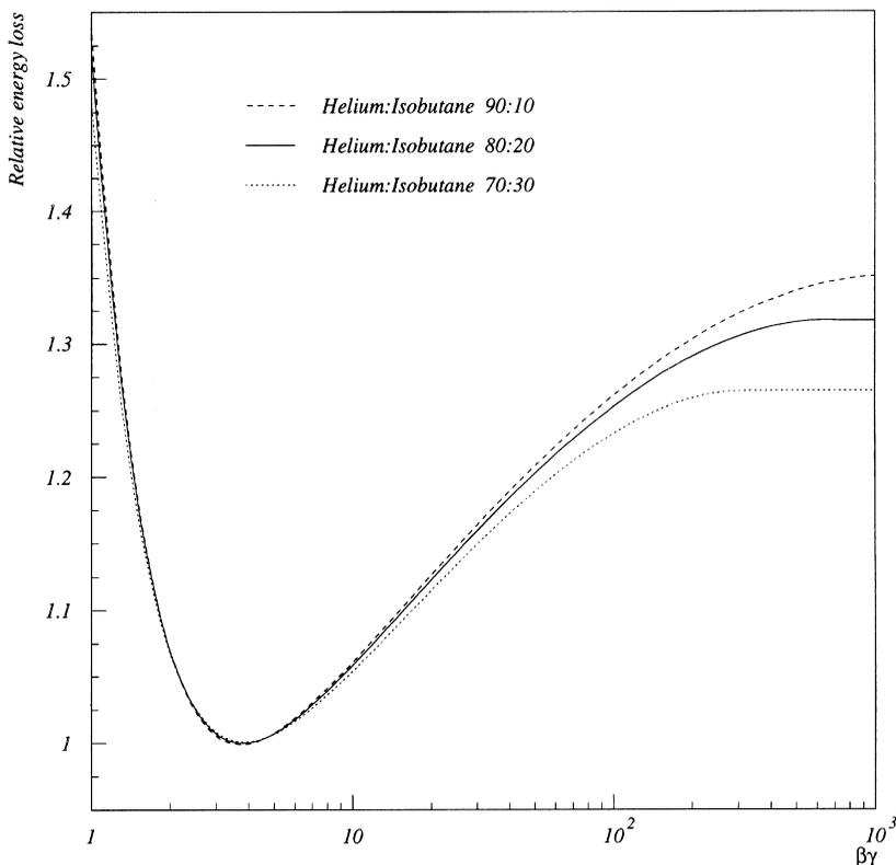
Fig. 7.  $dE/dx$  (arbitrary units) as a function of  $\beta\gamma$  for the three different He–Isobutane mixtures. 11 samples over 16.
