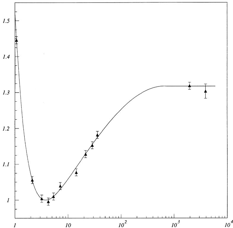
Fig. 6.  $dE/dx$  (arbitrary units) as a function of  $\beta\gamma$ . He–Isobutane 80:20. 11 samples over 16.
