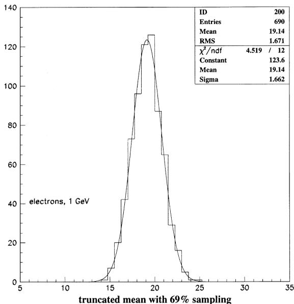
Fig. 5. Resolution in the measured  $dE/dx$  for 1 GeV/c electrons. He–Isobutane 90:10. 11 samples over 16.
