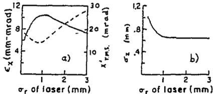
Figure 8. a) The transverse emittance  $\epsilon_x$ , (solid curve), and the r.m.s. beam divergence (dashed curve) as a function of the radius of the laser spot size on the cathode. b) The r.m.s. bunch length at the exit of the gun as a function of laser spot size. Other parameters are as in the table.
