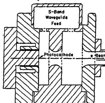
Figure 2. Section through the rf gun. Except for the waveguide feed the gun is axially symmetric. The 1 1/2-cells of the gun are 8 cm long.
