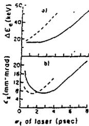
Figure 7. a) The beam energy spread  $\Delta E_e$ , and b) the transverse emittance  $\epsilon_x$  at the exit of the gun as a function of the laser pulse length. The solid (dashed) curves are for a peak rf field at the cathode of 100 (200) MV/m.
