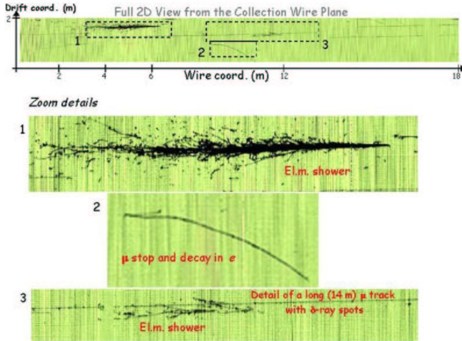
Figure 4: An event from the recent cosmic-ray test run of ICARUS [20], showing excellent track resolution over long drift distances in zero magnetic field.
