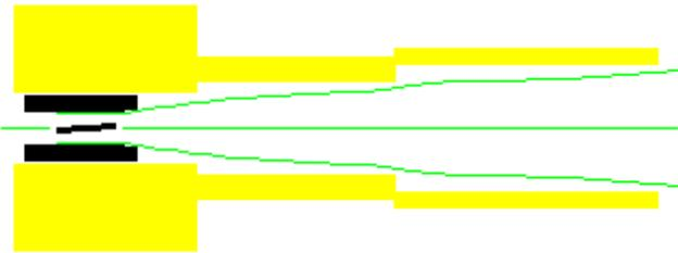
Figure 1: Pion-capture magnet, with average field  $B_0$  in target,  $-0.3 < z < 0$  meters. Magnet mass = 12 metric tons. 4 MW, 21 MJ outer set of coils energizes inner coil. Bore is ~0.15 m near target, ~0.6 m at mouth,  $z=L$ . For  $0 < z < L$ , the field profile ramps downward as  $B_0/(1+z/L)$ . The cone is the envelope of captured mesons.
