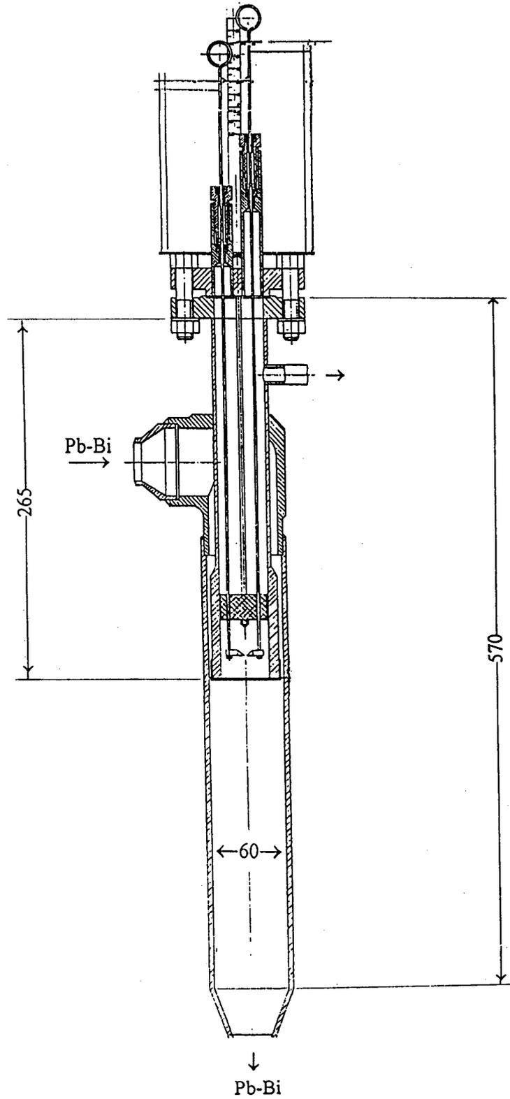
Fig. 3. Construction diagram of experimental model of liquid metal target.
