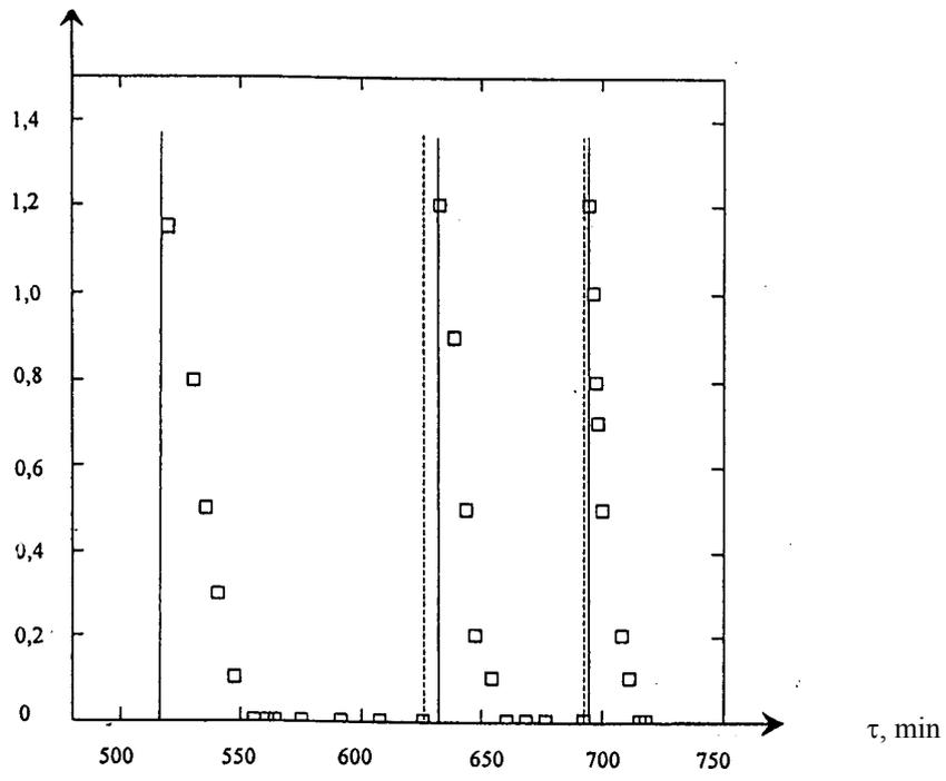
Fig. 2. Time dependence of gas pressure changing in the target cavity, caused by gas ejection by alloy flow.
