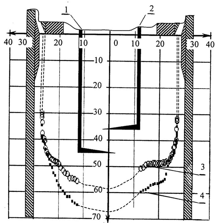
Fig. 4. Plane projection of the points of free surface profile of lead-bismuth coolant.
