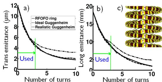
Figure 4: Simulation of a) transverse, & b) longitudinal, cooling in RFOFO 6D lattice; c) Cooling geometry.
