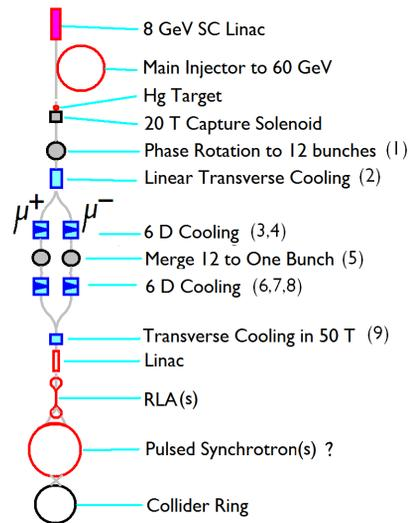
Figure 1: Schematic of Muon Collider components.
