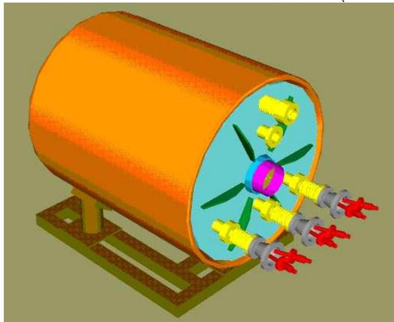
Figure 4: Sketches of the concept of a 15-T, pulsed copper solenoid for use in the prototype target studies [2].
