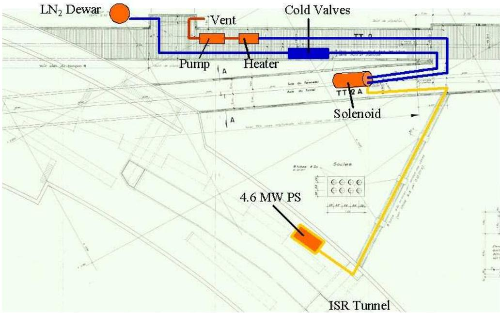
Figure 2: Plan view of a possible arrangement of DC power lines and the cryogenic transfers, with the solenoid magnet at the location of option 2. The 4.6 MW power converter could reside in the ISR tunnel, with the DC bussing passing through an existing 2-m high horizontal access shaft to the TT2A tunnel. The cryogenic transfer lines would pass along the TT2 tunnel and up the vertical access shaft to 6,000 l dewar on the surface.
