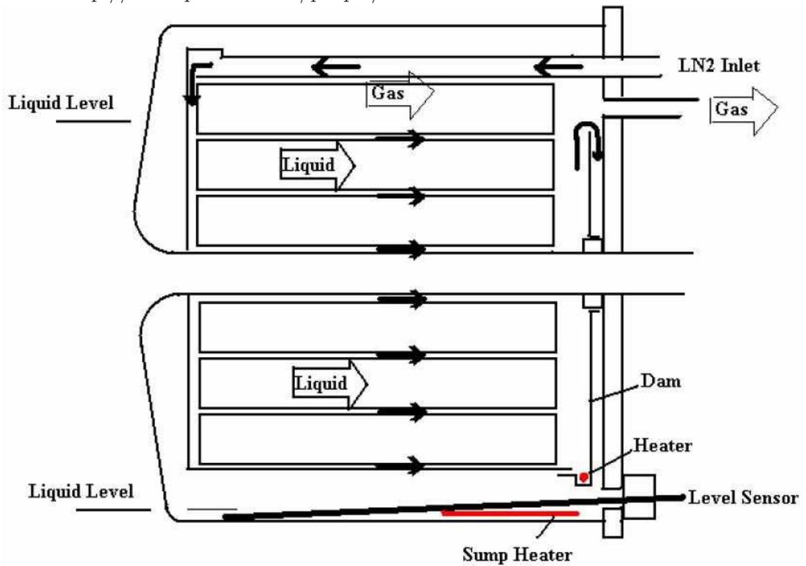
Figure 6: Sketch of the flow of liquid nitrogen within the magnet. From <http://198.125.178.188/bnlpulsed/dam.pdf>
