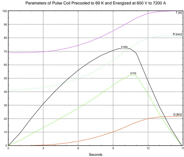
Figure 1: Time dependence in the 15-T pulsed magnet of the temperature  $T$ , the current  $I$  (with is directly proportional to the magnetic field  $B$ ), the coil resistance  $R$ , the voltage drop  $V$  across the coil, and the energy  $Q$  deposited in the coil by Joule heating.
