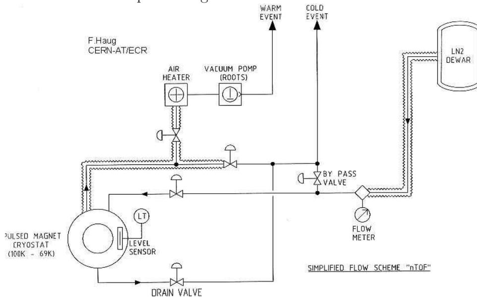
Figure 8: Sketch of a cryogenic system for operation of the magnet that uses the drain (F. Haug).
