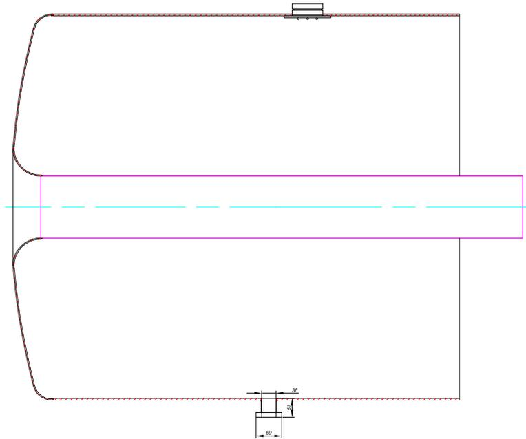
Figure 5: Vertical section through the outer vacuum vessel of the magnet, showing the drain port at the bottom. From drawing bnl-011.dwg, available at <http://www.psfc.mit.edu/people/titus>
