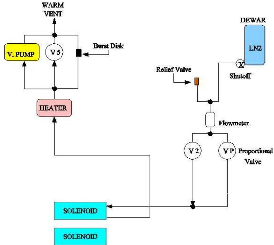
Figure 7: Sketch of a cryogenic system for operation of the magnet with an internal dam for the liquid nitrogen.
