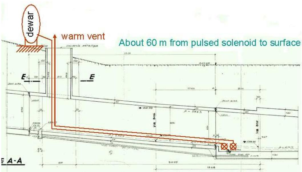
Figure 3: Elevation view of the sloping TT2 tunnel and the associated vertical access shaft. The cryogenic transfer lines are shown for option 1.
