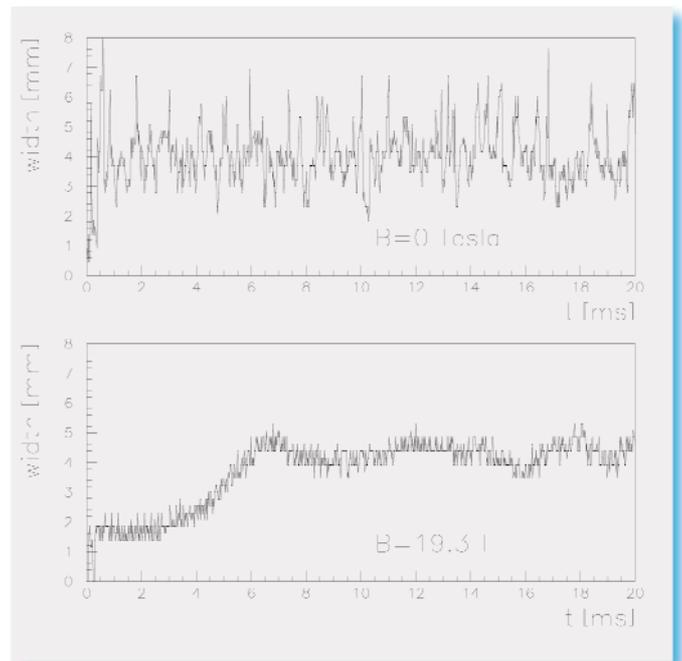
Figure 5.3: The width of the jet as a function of time at no magnetic field and at  $B = 19$  Tesla. A clear smoothing of the jet shape at 19.3 Tesla is visible.
