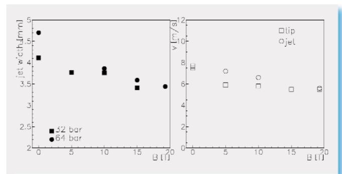
Figure 5.4: The pinching (left) and the velocity (right) of the jet as a function of the magnetic field strength. The decrease in the width is shown for two different driving pressures.
