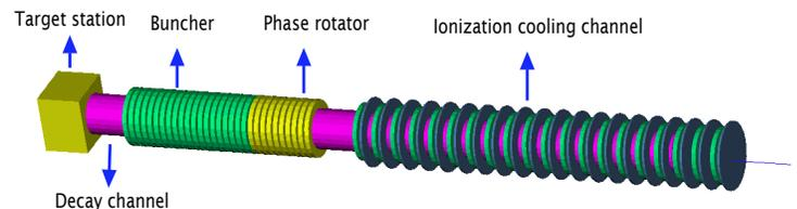
Figure 1: Schematic layout of the Muon Accelerator Front End based on [5].
