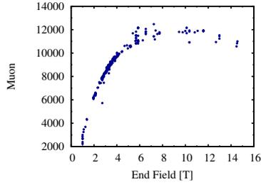
Figure 4: Dependence of the muon yield on the end field. Muons are counted at the end of Decay Channel.
