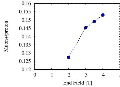
Figure 6: Normalized number of muons within the acceptance of the downstream accelerator as a function of the end field through the rest of the Front End.
