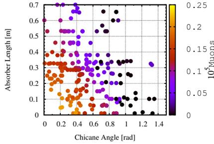
(a) Number of transmitted muons v.s. Chicane angle and absorber length.
