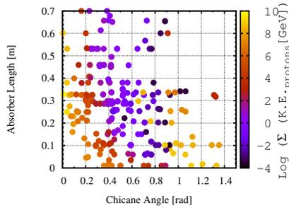
(b) Total transmitted K.E. after absorber v.s. Chicane angle and absorber length.
