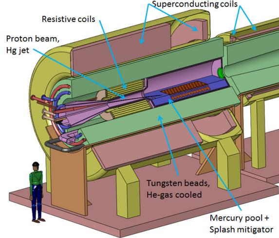
Figure 1: Neutrino Factory/Muon Collider Target System.
