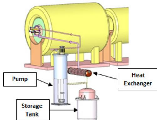
Figure 4: The external components of the mercury-flow loop.
