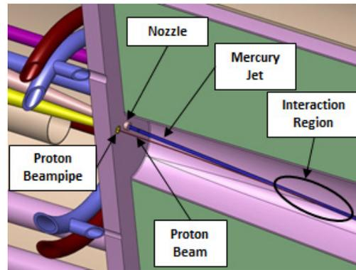
Figure 3: Interior of the Target Module showing the mercury nozzle and beam-entry pipe.
