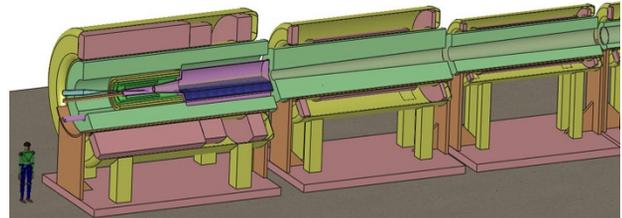
Figure 2: New layout of Neutrino Factory target station and capture solenoid. Due to engineering requirements the details of the layout of the superconducting coils have been changed to allow for room between the modules for maintenance. As the magnetic field profiles stayed unchanged so will the muon yield.
