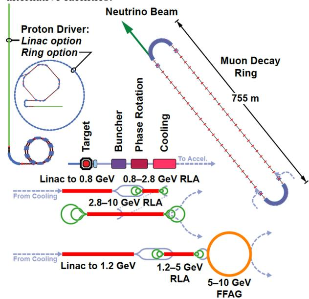
Figure 1: The accelerator facilities for the neutrino factory [2]. Compared to previous baselines the final muon energy has been reduced to 10 GeV following the Daya Bay and RENO results. Two different muon accelerator scenarios both derived from the previous baseline are under investigation to determine the most cost effective solution.
