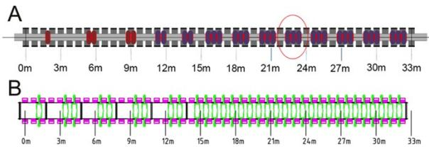
Figure 4: Changes to the buncher section due to engineering constraints. A shows the physics lattice design with one critical position marked. The highly modular engineering lattice adopted as baseline avoiding this problem is shown in B.
