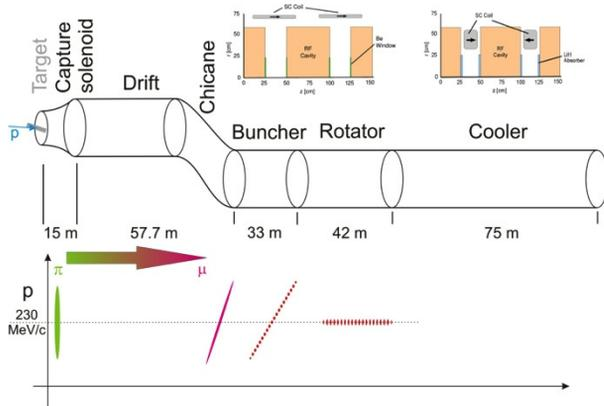
Figure 3: Schematic overview of the muon front end including the newly added chicane. The lattice design of Buncher, Rotator and Cooler are shown in the top row, while the bottom row shows the development of the particle burst within the front end.
