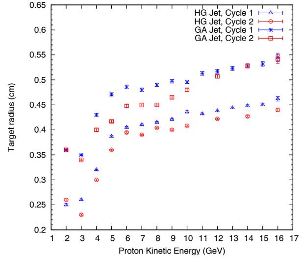
Figure 4: Optimized target radius as a function of proton kinetic energy.
