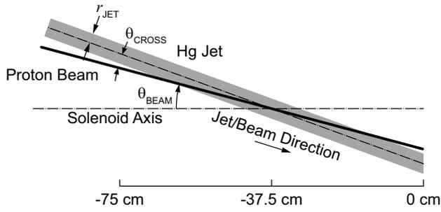
Figure 2: The mercury-jet-target geometry. The proton beam and mercury jet trajectories intersect at  $z = -37.5$  cm.
