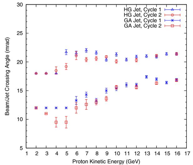
Figure 5: Optimized beam/jet crossing angle as a function of proton kinetic energy.
