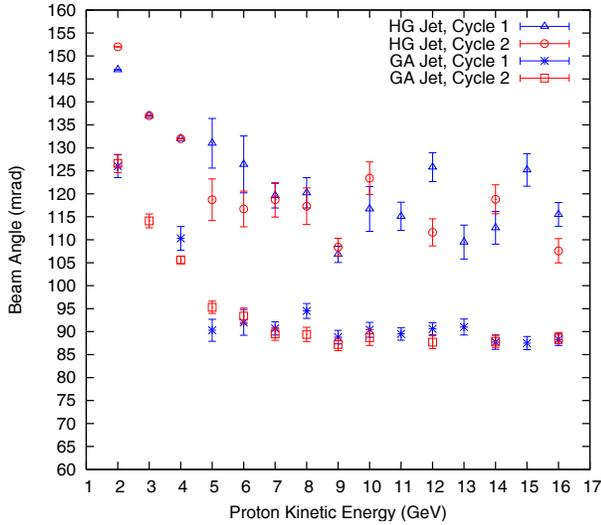
Figure 6: Optimized beam angle as a function of proton kinetic energy.
