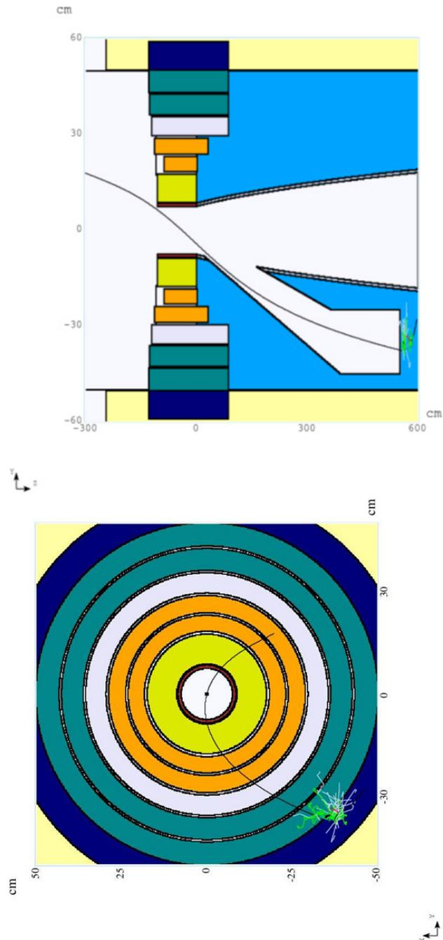
Figure 4: Top: Vertical ( $y$ - $z$ , top) and transverse ( $x$ - $y$ , bottom) projections of the (baseline) P12 proton-beam trajectory, neglecting interactions of the beam with the Hg target and pool.
