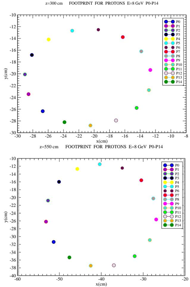
Figure 3: Proton-trajectory intercepts at  $z = 300$  cm (top) and  $z = 550$  cm (bottom) for 15 proton-beam configurations, each of which has the nominal beam/jet crossing angle at the center of the Hg target. The baseline configuration is that labeled P12.
