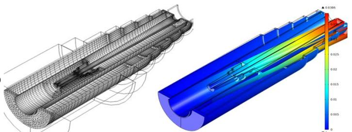
Above: Deformation  $\delta$ , magnified 20-fold, of the W-C shielding vessel When fixed only at its upstream end;  $\delta_{max} = 39$  mm
