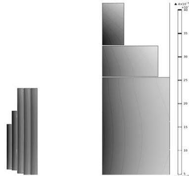
Above: Hoop strain  $\epsilon_0$  in resistive coils and SC coils #1-3. In all coils The maximum  $\epsilon_0$  is  $\sim 0.4\%$ ; in SC coil #1 it is 0.36%, implying a hoop stress of 720 MPa in the CICC conduit.
