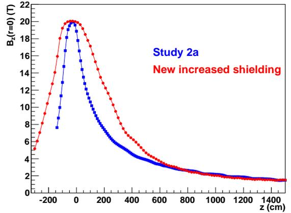
Figure 4: Comparison of the  $B_z$  magnetic field profile along the  $z$  axis for the Study 2a (blue squares) and the increased shielding (red circles) geometries.
