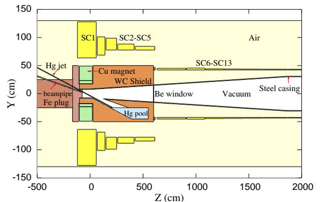
Figure 1: Schematic of the Study 2a target station geometry for the Neutrino Factory. The superconducting magnets are labelled SC $n$ , where  $n = 1$  to 13. The shielding consists of 80% tungsten-carbide and 20% water.
