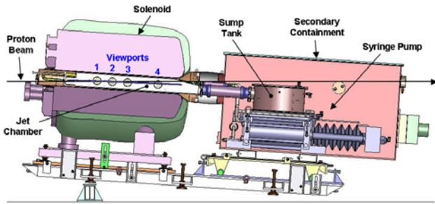
Figure 2: Cutaway side view of the MERIT experiment.
