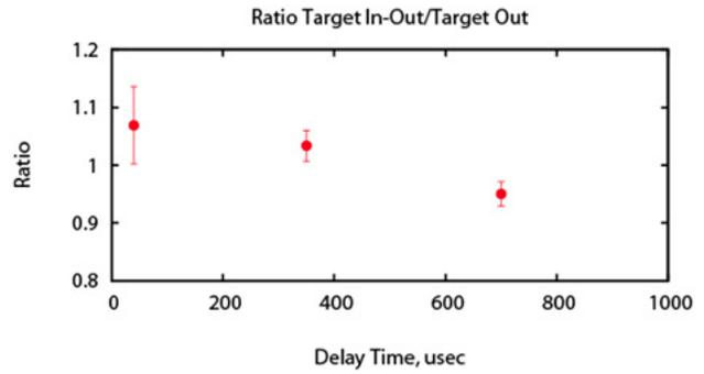
Figure 8: The probe/pump ratio for target-related particle production as a function of delay of the probe bunches.
