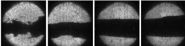
Figure 3: Images of jets with velocities of 15 m/s in magnetic fields of 0, 5, 10 and 15 T, without proton beam.
