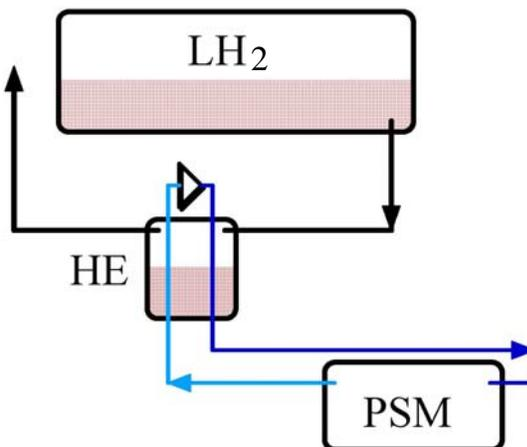
Fig. 2. Concept of the scheme to cool a pulsed solenoid magnet (PSM) by helium gas that is in turn cooled by liquid hydrogen ( $LH_2$ ) in a heat exchanger (HE).
