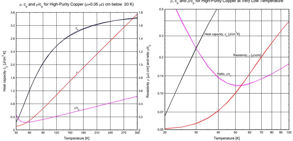
Fig. 1. Left: Electrical resistivity  $\rho$ , heat capacity  $c_p$ , and ratio  $\rho/c_p$  between room temperature and 30 K, for copper with a residual resistivity of  $0.05 \mu\Omega$  cm below  $\sim 20$  K. Right: Low-temperature electrical resistivity  $\rho$ , heat capacity  $c_p$ , and ratio  $\rho/c_p$  for copper with a residual resistivity of  $0.05 \mu\Omega$  cm below 20 K.
