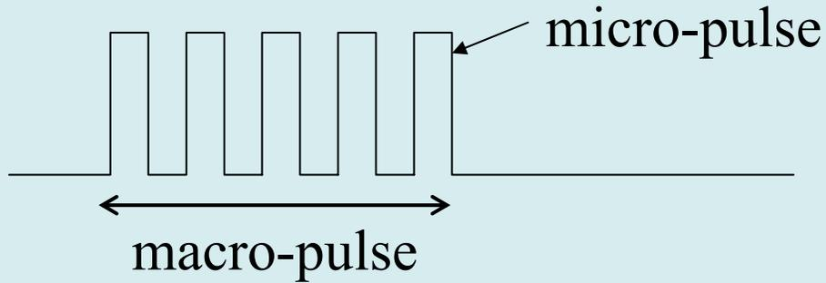
Proton beam "macro-pulses" and "micro-pulses".
