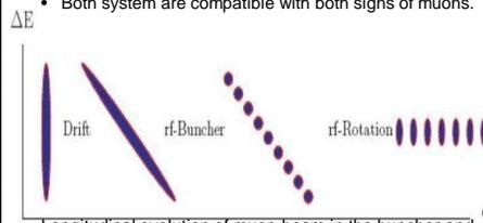
Longitudinal evolution of muon beam in the buncher and rotator.
