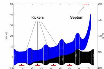
Layout of the baseline vertical/extraction system for the muon FFAG based on triplet cells
