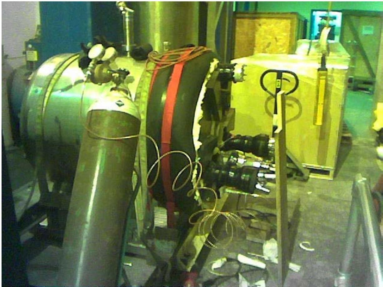
Pressure of 140 psi was applied – was not retained due to leaks in the Helium fill connections. Later when these were fixed, 93 psi was retained for 14 hrs. Helium bottle contents were not sufficient to go the 200 psi possible for the regulator. – Basically I ran out of Helium and didn't have time to get another bottle before shipping preparations were begun.
