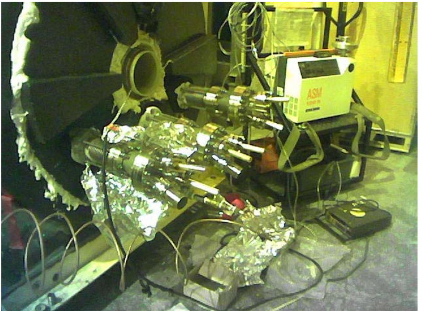
Pressure test setup with the helium leak detection system set up as a sniffer.
