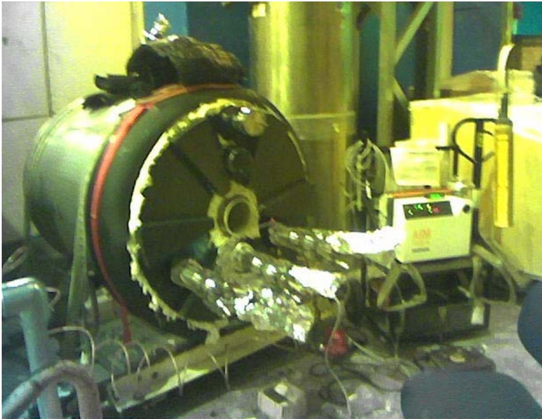
Aluminum foil was used to tent the joints to avoid contamination from the leak in the Helium gas inlet plumbing
