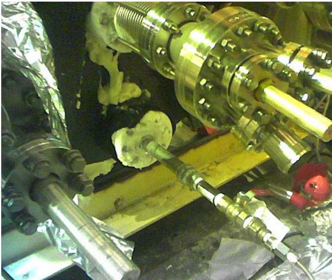
The close nipple was replaced with a pipe section with better formed threads. This did not leak
