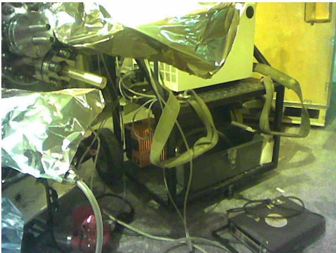
The sniffer probe was inserted in the aluminum foil tent around the joint being tested.
