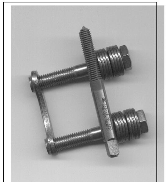
Platenut and Belleville stacks added to the packing nut/gland assembly
