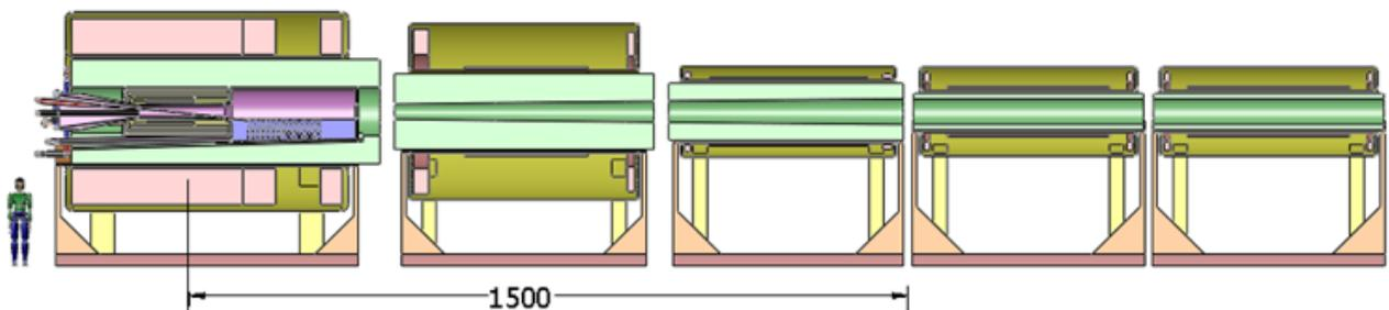
Figure 1: Vertical section of the three magnet modules of Target System (which nominally ends at  $z = 1500$  cm) and the first two modules of the Decay Channel.
