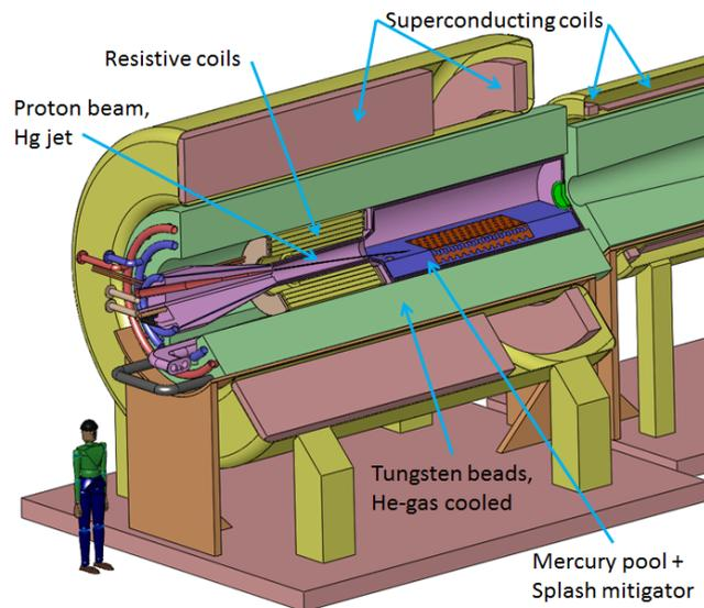
Figure 2: View of the 200-ton 20-T capture solenoid, with internal shielding by tungsten beads. The free-mercury jet target and the proton beam are tilted with respect to the magnetic axis, and impinge on the mercury-collection pool that also serves as the proton beam dump.
