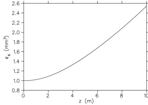
FIG. 3:  $\epsilon_6$  vs.  $z$  as calculated by ICOOL and reported by ECALC9 for a 10 m drift for a Gaussian beam. (color)
