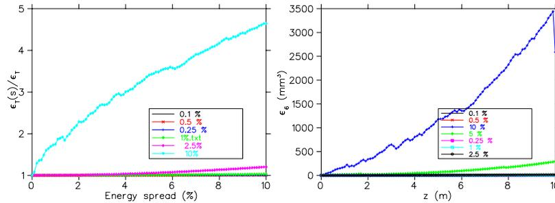
FIG. 4:  $\epsilon_T$  and  $\epsilon_6$  vs.  $z$  as calculated by ICOOL and reported by ECALC9 for a 10 m drift for a Gaussian beam; the different lines refers to different energy spreads. (color)
