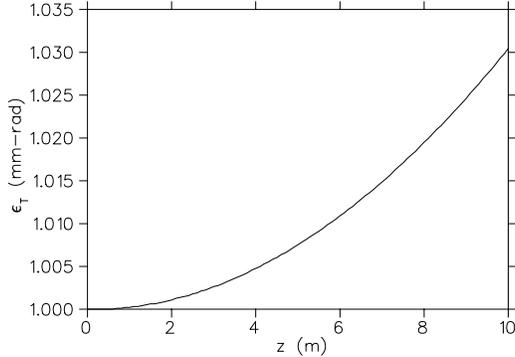
FIG. 2:  $\epsilon_T$  vs.  $z$  as calculated by ICOOL and reported by ECALC9 for a 10 m drift for a Gaussian beam. (color)
