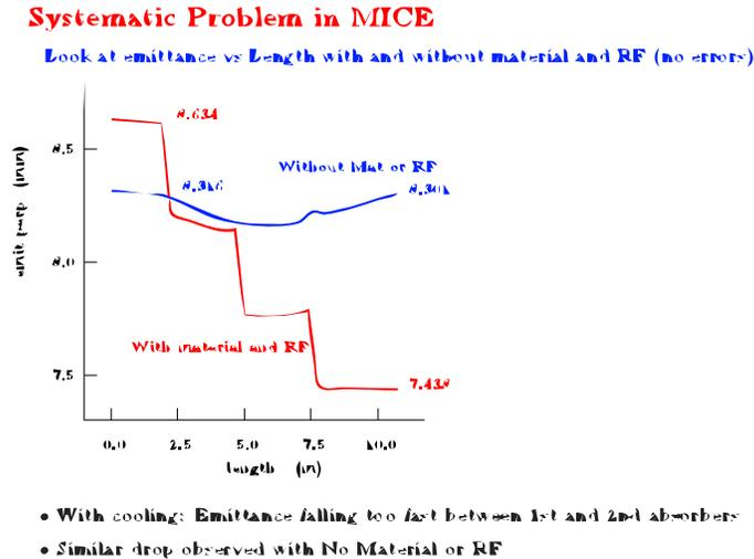
FIG. 1: MICE cooling channel. The transverse emittance does not remain constant in the region between the absorbers, as naively was expected. The superimposed curve depicts the emittance of the channel without material; both curves show similar behavior. (color)
