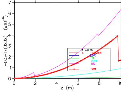
FIG. 5:  $I$  invariant vs.  $z$  as calculated by ICOOL and reported by ECALC9 for a 10 m drift for a Gaussian beam. (color)
