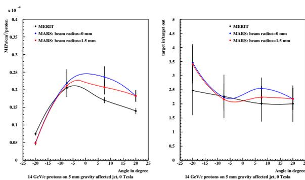
Figure 6: Left: The response of the pCVD diamond detectors installed at different angles around the mercury target for a 14 GeV/c proton beam compared to MARS simulation predictions. Right: The ratio of the response with and without the mercury jet for experimental data and simulations. The MARS simulation was done for a pencil like proton beam and for a beam with radius of 1.5 mm.
