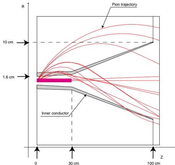
Figure 1: Pion trajectories for triangular horn shape
