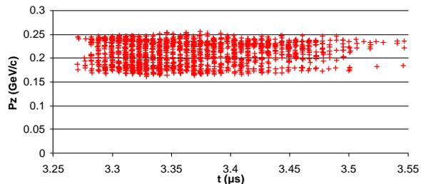
Figure 5. Output bunched beam, capturing from  $180 < P_z < 230$  MeV/c.
