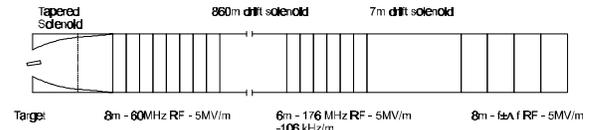
Figure 3. Scheme of the distributed RF capture system for a reduced muon momentum range. For final bunch momentum correction region,  $f=174.6219$  MHz – 0.106 MHz/m and  $\Delta f=1.4543$  MHz. The region to the left of the dashed line was modelled with FLUKA.
