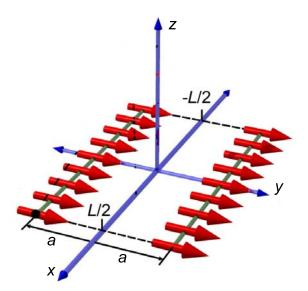
Trapping in the horizontal (x-y) plane is provided by the magnetic field, but the field alone does not provide trapping in the vertical (z) direction, where a combination of gravity and magnetism can give trapping. The latter is a bit subtle, in that the vertical equilibrium
