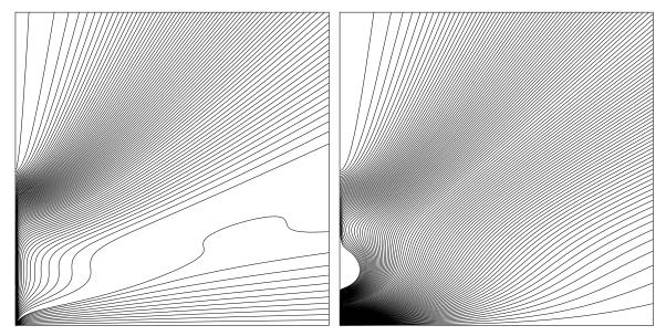
The plots on the next page show lines of the electric field at time t=0 (left) and  $t=\pi/2\omega$  (right) for the uncut,  $3\lambda/2$  dipole antenna.<sup>7</sup>
