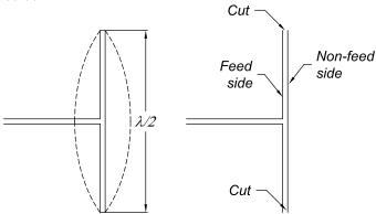
One of us (DJJ) has performed an experiment with a half-wave<sup>2</sup> folded dipole antenna [3], which has current nodes at the ends of the antenna according to eq. (2), as shown in the left of the figure above. However, the radiated power from the cut antenna (above right) was much less than that of the uncut antenna, as shown in the Smith charts [4] below.
