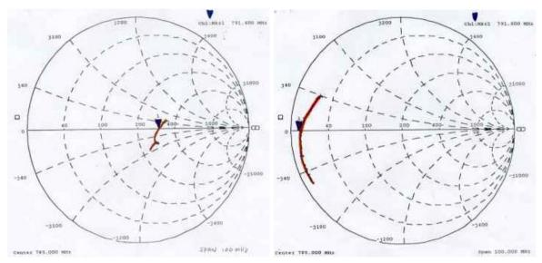
The radiation resistance of the whole antenna was about 300  $\Omega$ , as determined by an HP8714C network analyzer, while that of the cut antenna was only a few ohms. The resonant frequency of both the uncut and cut antennas was 790 MHz, the total length of the antenna conductor (feed side + non-feed side) was 32 cm, and the frequency scan was from 735 to 835 MHz.
