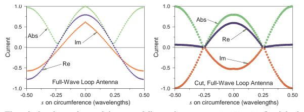
The calculated impedance of the uncut full-wave loop antenna is  $122 - 95i \Omega$ , while that of the antenna after is has been cut at  $\pm 90^{\circ}$  from its feedpoint is  $103 + 91i \Omega$ . In this example,
