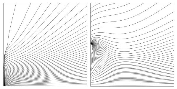
Since the antenna is assumed to be made of perfect conductors, there can be no tangential electric field at the surface of the antenna, and consequently no lines of the Poynting vector,  $\mathbf{S} = \mathbf{E} \times \mathbf{H}$ , can emanate from the antenna conductors. Rather, the lines of the Poynting vector all emanate from the feedpoint of the uncut antenna (above left), and the conductors of the antenna serve to guide those lines through the near zone into the far zone.
