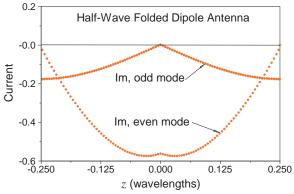
We see from the righthand figure on the bottom of p. 2 that cutting the antenna at its ends results in a substantial perturbation to the current, whereby the imaginary part of the current becomes much larger than the real part, and we cannot expect the radiation of the cut antenna to be the same as that of the uncut case. The imaginary part of the current is now almost entirely in the "odd" mode, while the tiny real part of the current is a mixture of "even" and "odd" modes.
