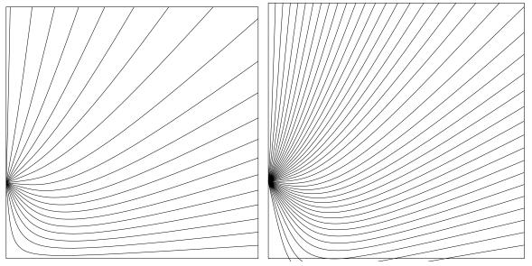
The plots below show lines of the magnetic field at time t=0 (left) and  $t=\pi/2\omega$  (right) for the uncut, full-wave loop antenna.
