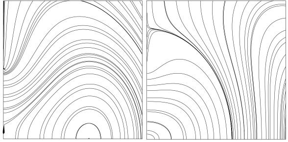
Note that the lines of  $\mathbf{E}$  emerge from the antenna (which lies along the lower half of the left edge of the plots above) at right angles to the surface of the conductor, as required for good/perfect conductors.
