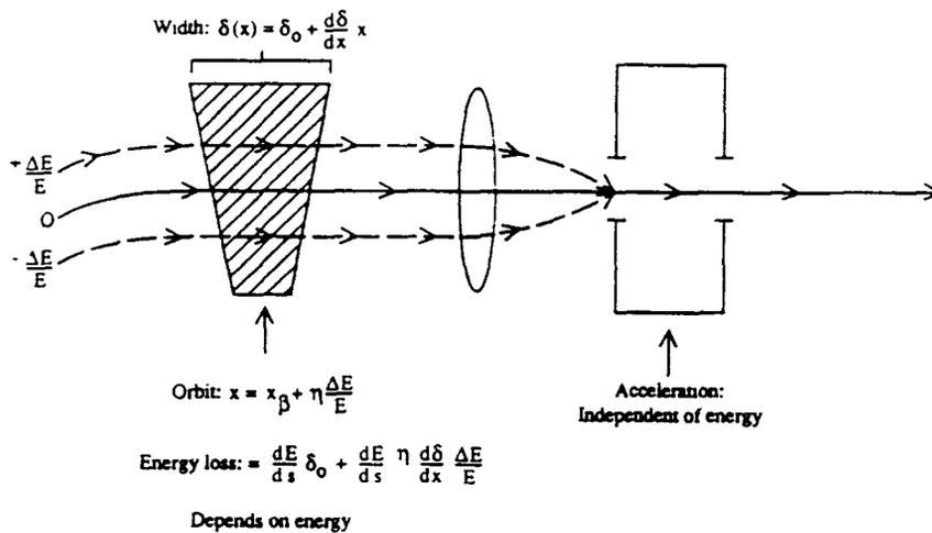
Fig. 4. Enhancement of energy cooling by using a wedge absorber placed in a non-zero dispersion region. The thickness of the absorber depends on transverse position ( $\Delta = \delta_0 + (d\delta/dx)x$ ), and the position at the absorber depends on the energy ( $x = \eta(\Delta E/E)$ ), producing an enhanced energy dependence of energy loss, decreasing energy spread. Energy recovery in the accelerator is independent of energy. (Transverse cooling decreases with enhanced energy cooling.)
