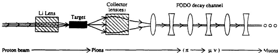
Fig. 2. Schematic view of  $\mu$ -production from  $\pi$ -decay, with  $\pi$ 's produced from hadrons. A high-energy hadronic beam is focused onto a target; a collector lens(es) collects the resulting  $\pi$ 's into a strong-focusing “FODO” channel, where  $\pi$ -decay produces  $\mu$ 's for collider use.
