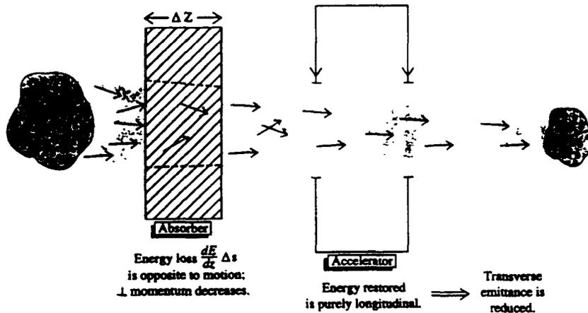
Fig. 3. Schematic view of transverse "ionization cooling". Energy loss in an absorber occurs parallel to the motion; therefore transverse momentum is lost with the longitudinal energy loss. Energy gain is longitudinal only; the net result is a decrease in transverse phase-space area.
