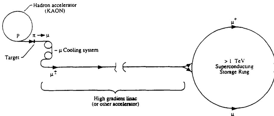
Fig. 1. Overview of linac-based  $\mu^+ - \mu^-$  collider, showing a hadronic accelerator, which produces  $\pi$ 's on a target, followed by a  $\pi$ -decay channel ( $\pi \rightarrow \mu\nu$ ) and  $\mu$ -cooling system, followed by a  $\mu$ -accelerating linac, feeding into a high-energy storage ring for  $\mu^+ - \mu^-$  collisions. (The linac could be replaced by a rapid-cycling ring; see Fig. 6.)
