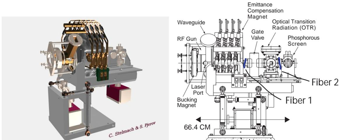
Figure 1: Drawings of the BNL ATF rf gun. Two 30-cm-long BCF-12 scintillating fibers were placed on the output side of the gun, just upstream of the gate valve, and just upstream of the phosphorous screen.
