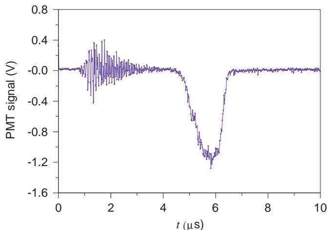
Figure 3: The observed PMT voltage *vs.* time from the x-ray signal in fiber 1 at a peak electric field of 110 MV/m in the rf cavity.
