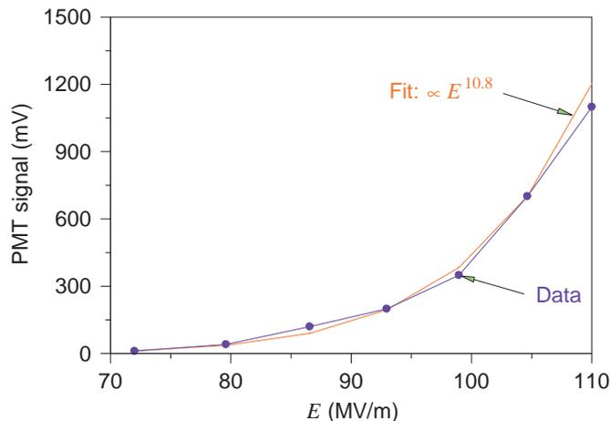
Figure 2: The observed PMT voltage from the x-ray signal in fiber 1 as a function of the peak electric field in the rf cavity, with the electron beam off and the compensating solenoid off.
