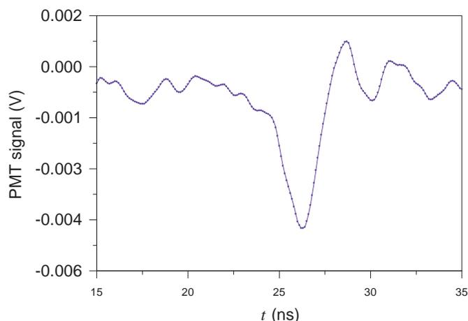
Figure 4: A single photoelectron signal in the PMT at 1680 V.
