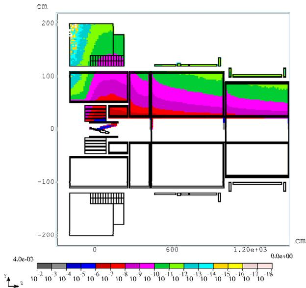
Figure 3: Simulated power deposition in the Target System for a 4-MW proton beam, averaged over azimuth.
