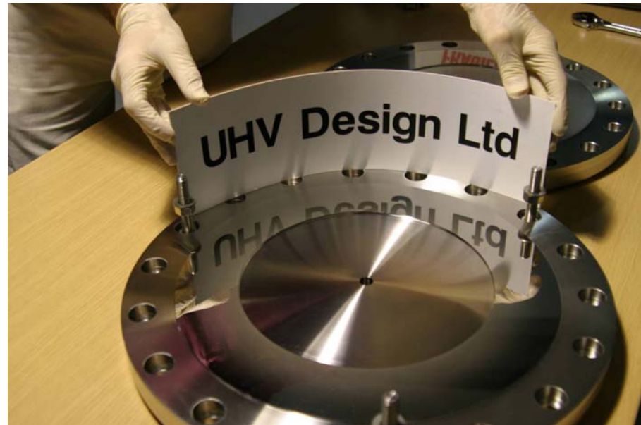
Polished flange (surface roughness, R_a = 0.020 \mu\text{m} )
