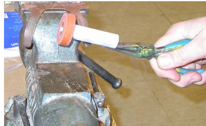
LN2 Dunk Test: Feb 9 2006 The gland for the power lead did not shatter – but it was rigid.
