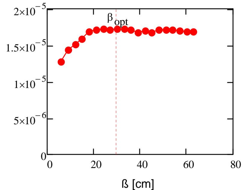
*Graphite cylind. target, backward muons,  $p_{\text{prot}}=2\text{ GeV}/c$ ,  $\varepsilon_x=\varepsilon_y=1\text{ cm}$ ,  $\Delta p/p=\pm 0.15$ ,  $\theta=200\text{ mrad}$ ,  $B=2.5\text{ T}$*
