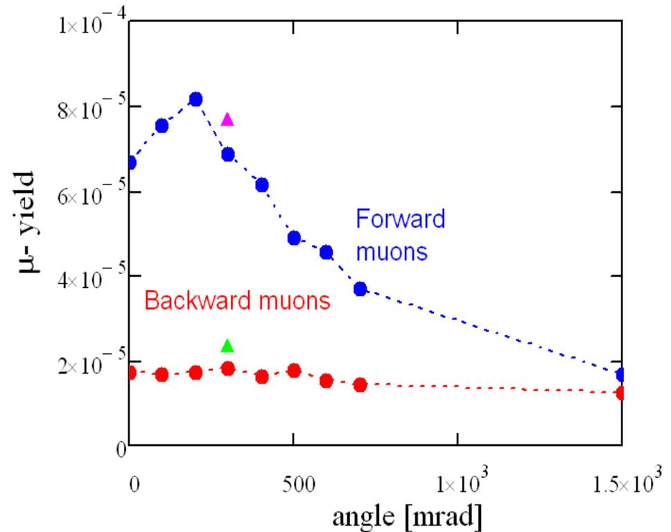
*Dependence of muon yield on the target angle relative to magnetic field for carbon target into the following phase space:  $\varepsilon_x = \varepsilon_y = 1$  cm,  $\Delta p/p = \pm 15\%$ ,  $p_{\text{prot}} = 3$  GeV/c, ( $E_{\text{kin}} = 2.21$  GeV)
