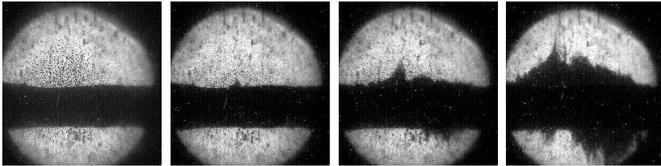
Fig. 6. A 1-cm diameter, 15-m/s Hg jet at 0, 75, 175, and 375  $\mu\text{s}$  after interaction with  $10 \times 10^{12}$  24-GeV protons in a 10-T solenoid field.
