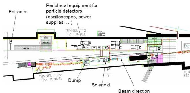
Fig. 1. The experimental setup in the TT2/TT2A tunnels of CERN PS. The beam arrives from the right side of the figure and after traversing the experiment is stopped in an iron dump before reaching the nTOF target shown on the left.
