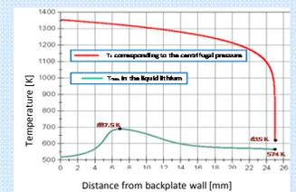
$T_{max}$  and  $T_{sat}$  at beam footprint lower edge
