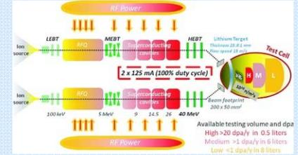
IFMIF scheme of main facilities: Linear Accelerator; Lithium Target; Test Cell
