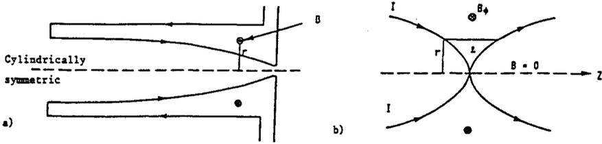
**Figure 2a, b:** The current profile and parabolic magnetic field shape in a typical parabolic horn, from reference [1].
