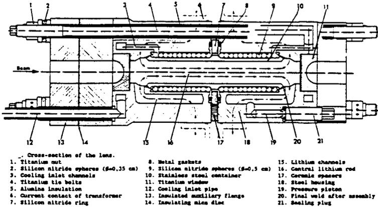
**Figure 4.** Lithium lens from CERN, from reference [5]. © 1985 IEEE
