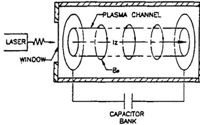
**Figure 8.** Schematic of a plasma channel (spark- or Z- channel) which may be adaptable as a lens for a muon collider [10].
