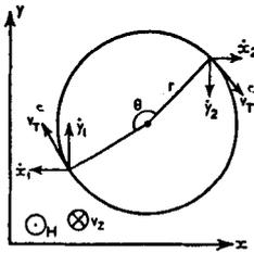
**Figure 6a:** Geometry of the the transverse motion of a charged particle in the uniform field of a solenoid , from reference [8] .
