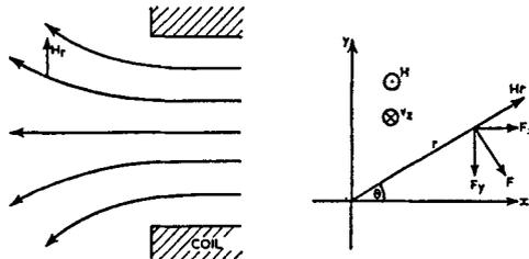
**Figure 6b:** Geometry of the the fields and forces on a charged particle at the end of a solenoid (axial view), from reference [8] .
