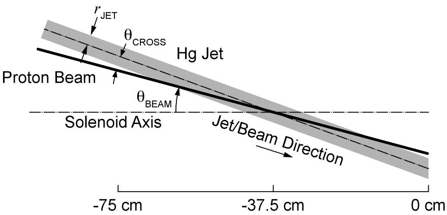
Hg Jet is replaced by vacuum for tracking of single proton from z=-75 cm to z=-37.5cm. The Initial position of x0 and y0 at z=-75 cm is adjusted for the launched single proton with specified Ekin and beam angle to make sure the (x, y) of single proton at z=-37.5 cm to be (0,0).
