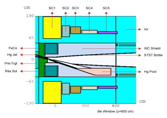
Concept of a continuous mercury jet target for an intense proton beam. The mercury jet is tilted by 100mrad with respect to a 20-T solenoid magnet which captures and conducts low-momentum pions into a decay channel.
