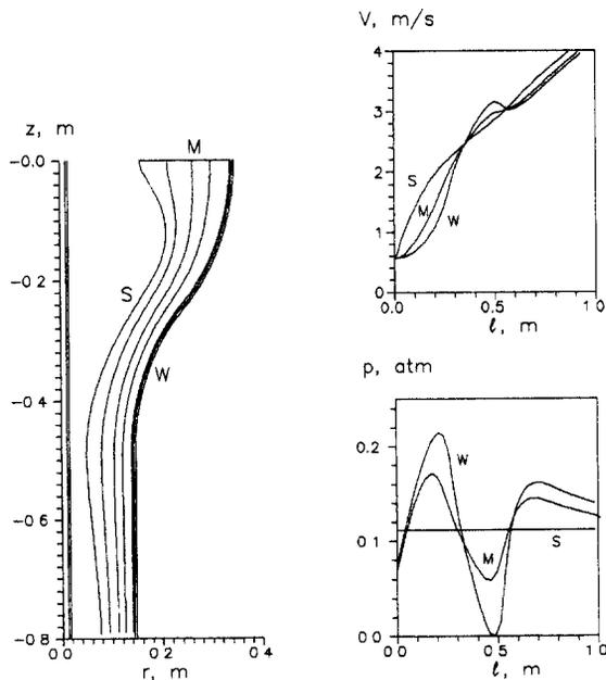
Fig. 3. The stream line configuration, the pressure ( $p$ ) and velocity ( $V$ ) for the "hole" flow regime.
