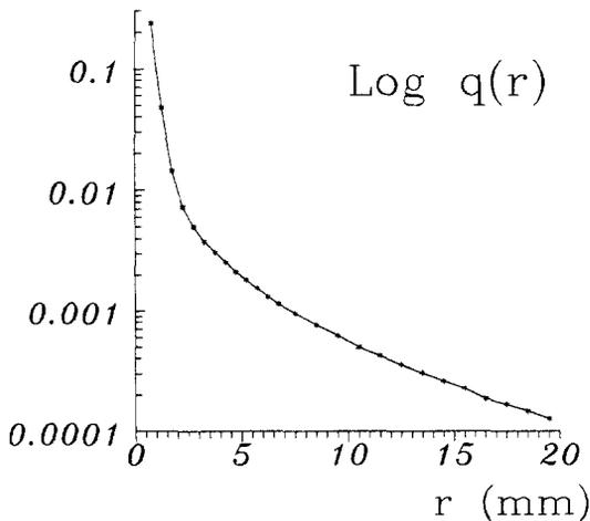
Fig. 1. The radial heat deposition in the lead–bismuth medium under the thickless proton beam operation.
