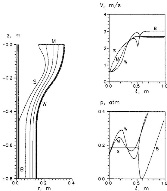
Fig. 5. The stream line configuration, the pressure ( $p$ ) and velocity ( $V$ ) for the “whole” flow regime by normal the eutectic consumption.
