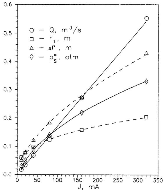
Fig. 6. The eutectic consumption ( $Q$ ), the lower target’s dimension ( $r_1$ ), the upper target’s dimension ( $\Delta r$ ) and the minimal pressure over free surface ( $p_s^*$ ) for the flowing heavy metal targets within the 10–320 mA proton current ( $J_b$ ) range.
