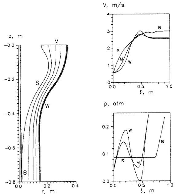
Fig. 4. The stream line configuration, the pressure ( $p$ ) and velocity ( $V$ ) for the "whole" flow regime by minimal the eutectic consumption.
