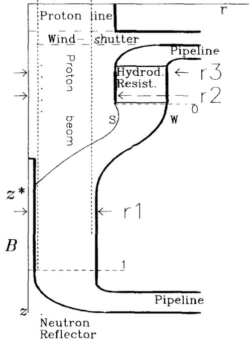
Fig. 2. The scheme of a flowing heavy metal target for an accelerator-driven neutron source.
