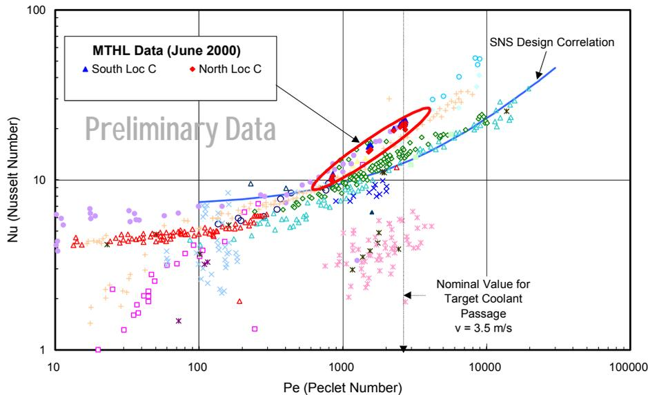
Figure 3. Heat transfer data from MTHL agrees with design correlation predicted from CFD calculations.
