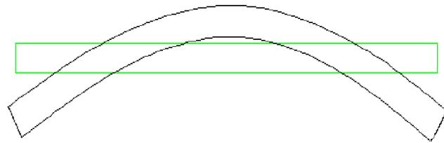
Fig. 6. Deformed shape at 12 ms (10000x) show bending mode character.
