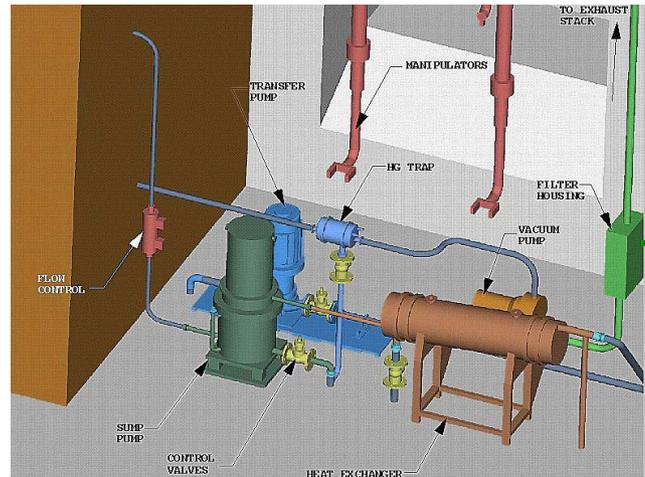
Figure 5: Hot cell arrangement for the mercury target equipment.
