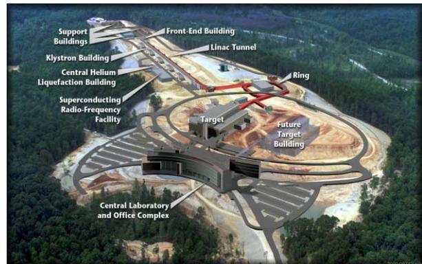
Figure 1: The site layout of the Spallation Neutron Source in Oak Ridge, Tennessee.
