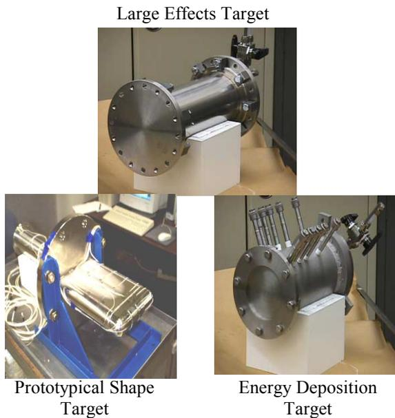
Figure 4: Target modules used in the WNR tests for pressure wave analysis.
