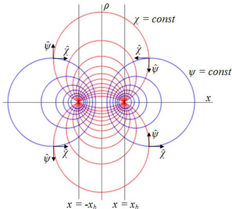
The electric field lines (but not the scalar potential) for  $x > -ct$  lie on surfaces of constant coordinate in a bipolar coordinate system with foci at  $x = \pm x_b(t)$ , illustrated in the figure
