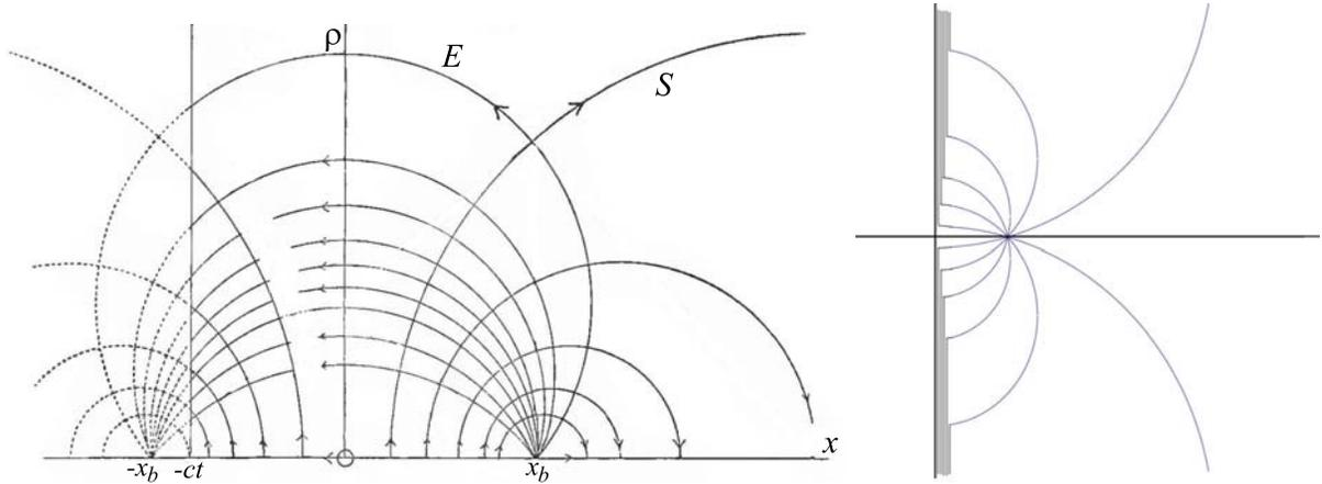
In the plane  $x = -ct$ , where the potentials (32) are singular, the fields are those of a singular wavefront,
