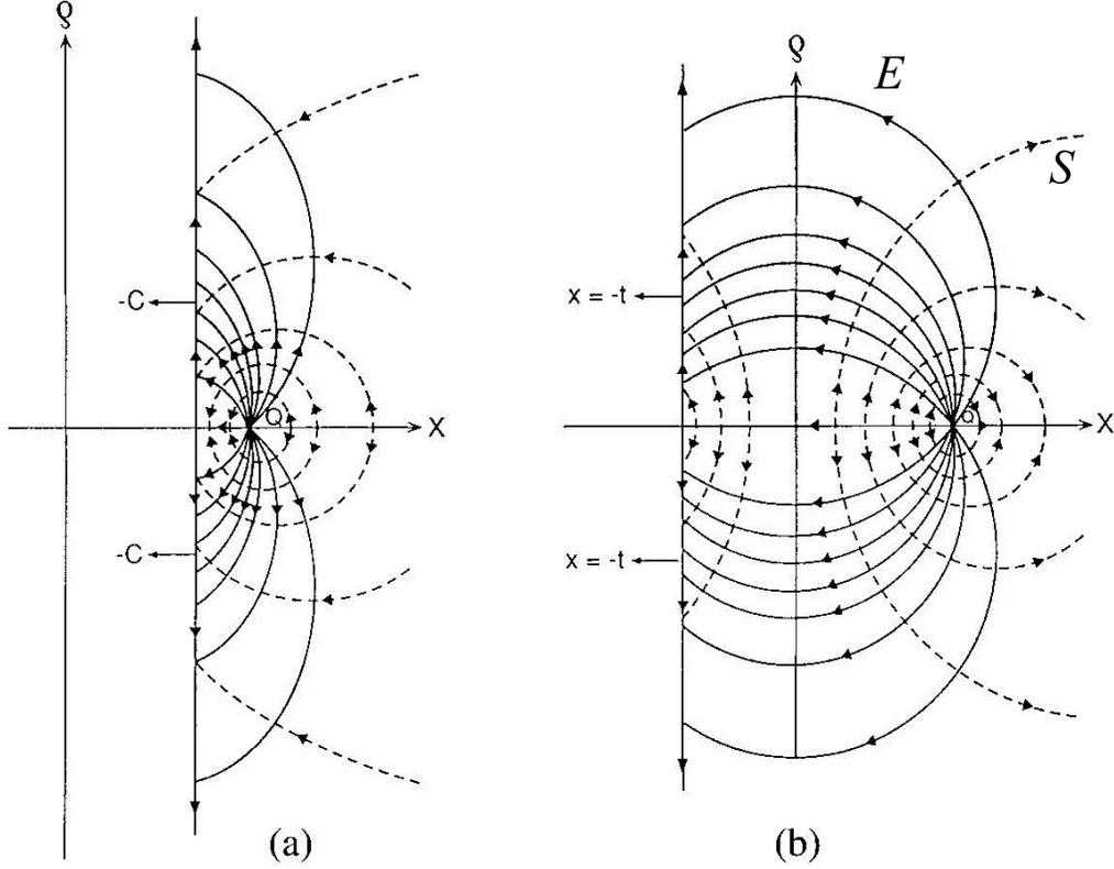
The figures suggest that the fields close to the charge resemble those of a uniformly moving charge, while away from the charge they curve towards the image charge at  $x = -x_b$ . This will be verified in sec. 2.4.
