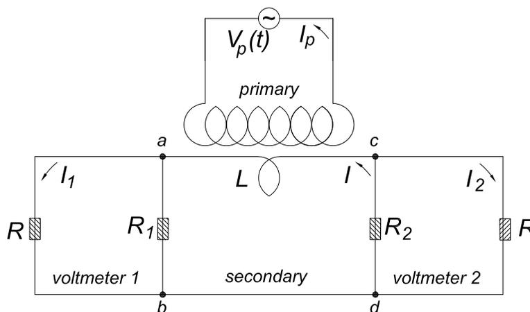
Kirchoff's loop equation for the central (secondary) loop in Lewin's example is,<sup>8</sup> for the secondary loop is,
