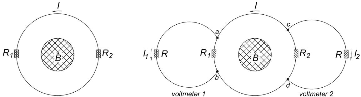
This circuit is probed by two voltmeters as sketched in the righthand figure above. Each voltmeter consists of a resistor  $R \gg R_1, R_2$  and an ammeter that measures the currents  $I_i$  and reports the “voltage”  $V_{\text{meter},i} = I_i R$ .<sup>5</sup> The “positive” leads of the voltmeters are connected to points  $a$  and  $c$ , such that the directions of currents  $I_1$  and  $I_2$  are as shown when positive.
