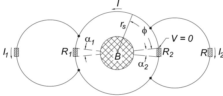
Resistor  $i$  has resistance  $R_i = r_s \alpha_i / \sigma_i A_i$ , where  $\alpha_i$  is its azimuthal extent,  $A_i$  is its cross-sectional area, and  $\sigma_i$  is its conductivity. The current in each resistor  $R_i$  is  $I$  to a good approximation (since  $I \gg I_1$  and  $I_2$ ), so the current density is  $J_i \approx I/A_i$ , and Ohm's law can be written as,
