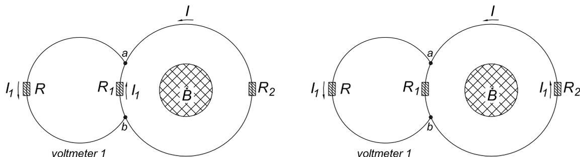
Hence, the value of the current  $I_1$  does not depend on whether it flowed on the left or on the right side of the primary loop, and the circuit analysis based on Kirchoff’s law cannot determine the partitioning of current  $I_1$  between the left and right sides.
