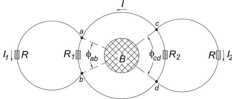
Only if the meter leads were connected directly to the ends of resistors  $R_1$  and  $R_2$  (as would be good practice), and the resistor have negligible azimuthal extent, would the meter readings (8) equal the voltage differences (differences in the electric scalar potential) between the tips of the leads.<sup>16,17</sup>
