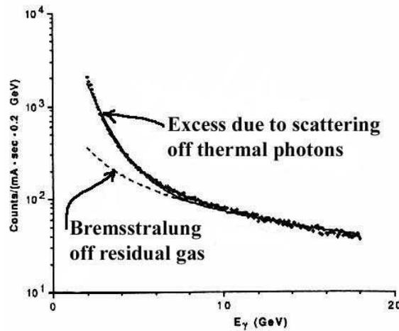
Figure 4. Scattering of 50-GeV electrons off the “vacuum” includes a signal of bremsstrahlung due to residual gas molecules, as well as “inverse” Compton scattering off thermal photons.<sup>13</sup>
