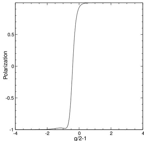
Figure 5. Calculated dependence of the residual polarization in an electron storage ring on the  $g$ -factor of the electron.<sup>25</sup>
