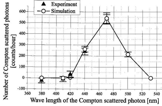
Figure 10. The wavelength of second harmonic scattering in the collision of an 800-nm Ti:sapphire laser of strength  $\eta = 0.6$  with a 10-keV electron beam is shifted from 400 nm to 470 nm due to the large effective mass  $\bar{m} = m\sqrt{1 + \eta^2}$  of the electron inside the laser beam.<sup>42</sup>
